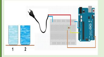
$\cdot$  One pin of the power cable will be connected to Arduino's GND pin and the other pin to Arduino's A0 pin.
